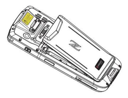
Step 2: Gently push the SD/SIM card into the card holder (please pay attention to the direction of the notch when inserting the card)
